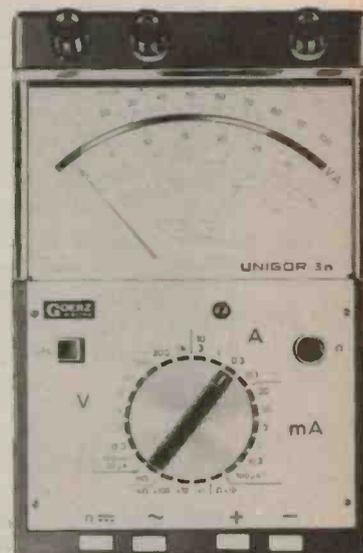
The push-button polarity-reversal switch of the Unigor 3n simplifies the testing of semiconductors.
